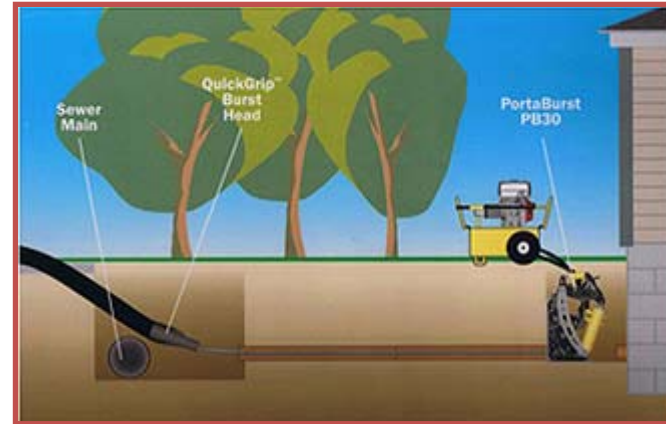
EXAMPLE of a trenchless repair
